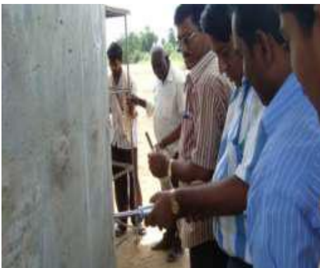
Fig 8 : Testing of Bridge Pier using Rebound Hammer
